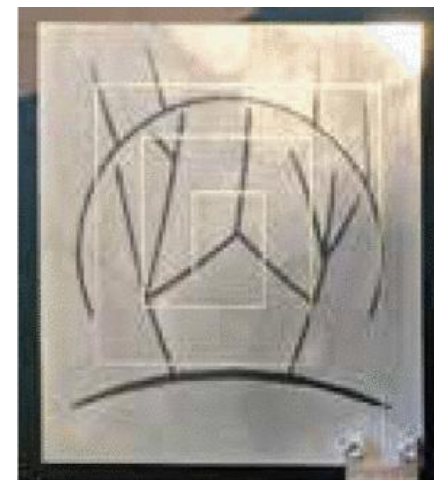
Figure 5 – Slot antenna design created to mimic the veins in the human hand. [2]
