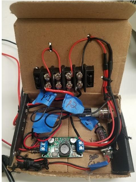
Figure 2.10: Fabricated power supply circuit which contains the UBEC and the DC-to-DC converter as well as the toggle switch for turning on the device.
