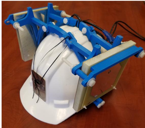
(b) Two RFID antennas mounted on helmet
