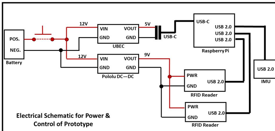
Figure 2.11: Electrical schematic for the power supply to all devices as well as the USB connections required to control all devices.
