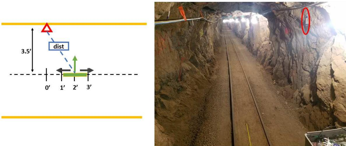
Figure 3.3: Second measurement scenario to create data for the look-up-table. The diagram on the left shows the setup of the measurement. The distance used for the look-up-table is the length from the center of the tag to the center of the antenna. The red triangle represents the RFID tag and the green rectangle represents the antenna. The right picture shows the location of the tag for this measurement. The red oval is the location of the tag under test.
