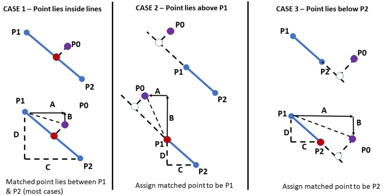
Figure 3.19: The three possible scenarios when matching a point to curve; figure modified from the one shown in [47].  $P0$  is the point that is being matched.  $P1$  is the starting coordinate of a line segment.  $P2$  is the end coordinate of a line segment.  $A, B, C, D$  are geometric quantities used in the map matching code. The red dot is the map matched point. The white dot shows where the point would have projected to if the line extended to infinity. See Listing C.16
