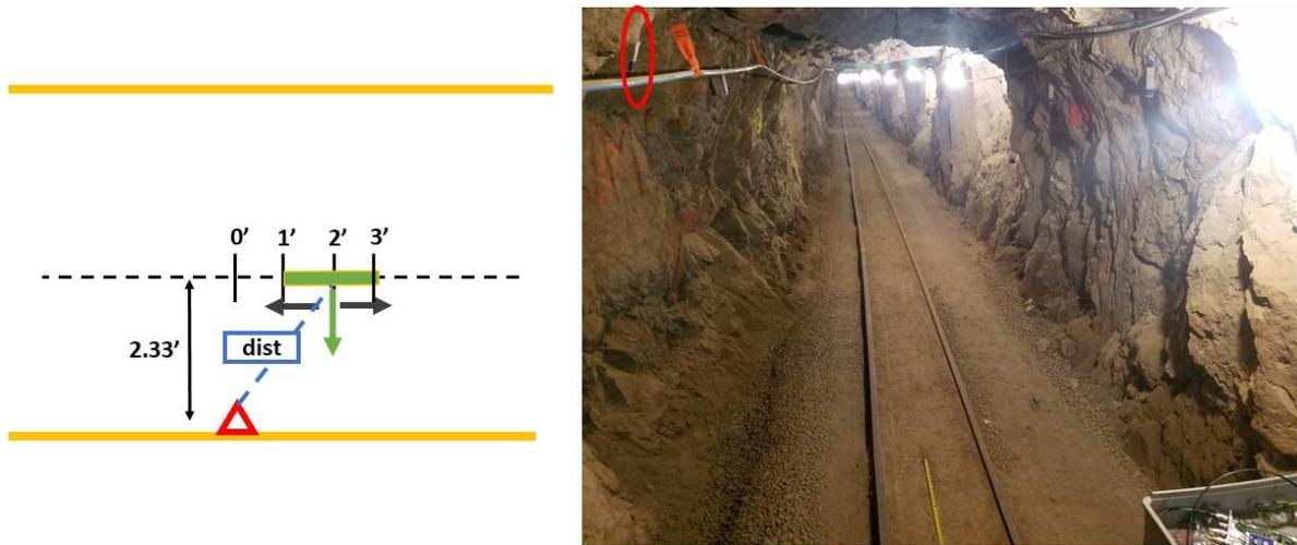
Figure 3.4: Third measurement scenario to create data for the look-up-table. The diagram on the left shows the setup of the measurement. The distance used for the look-up-table is the length from the center of the tag to the center of the antenna. The red triangle represents the RFID tag and the green rectangle represents the antenna. The right picture shows the location of the tag for this measurement. The red oval is the location of the tag under test.
