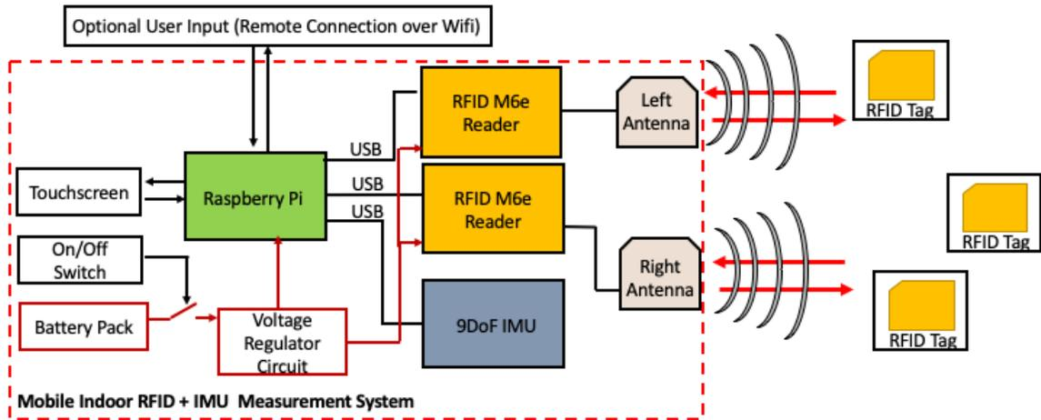
Figure 2.1: Hardware block diagram of the localization prototype.
