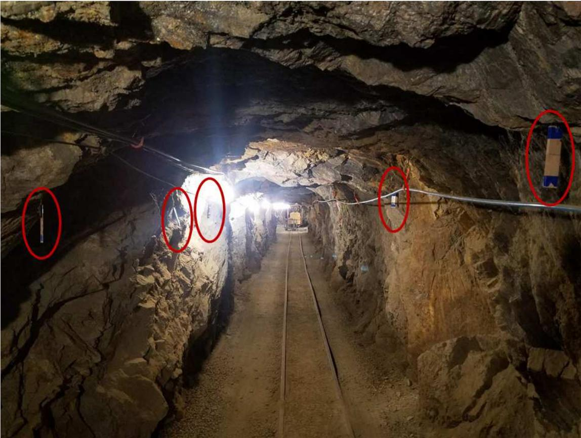
Figure 4.4: Picture of zone 1; an exemplary straight section. The red ovals highlight the tags in view.
