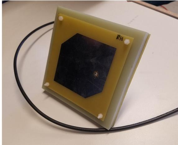
(a) Right-hand circularly polarized RFID antenna
