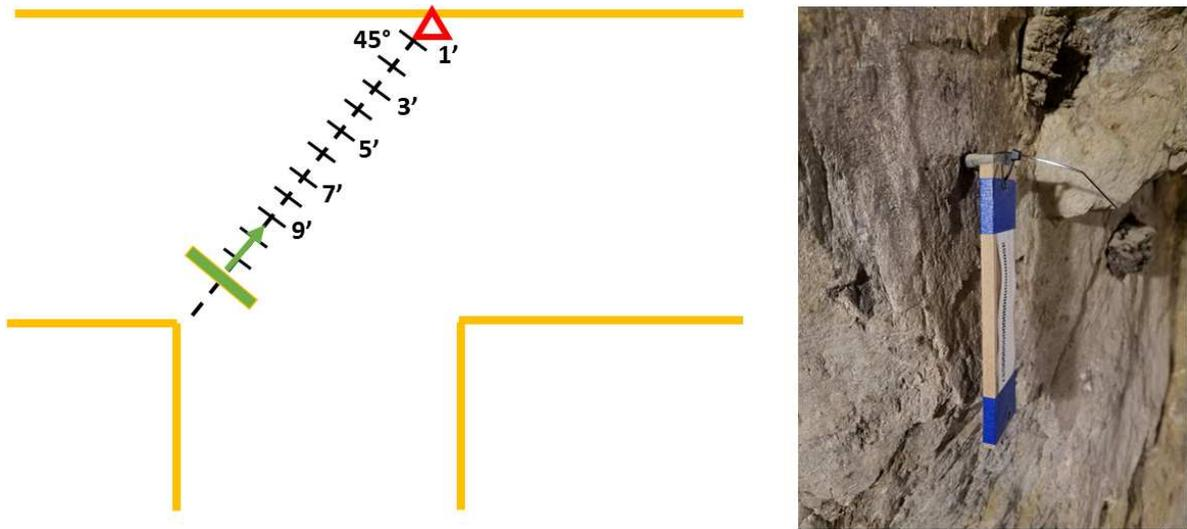
Figure 3.2: First measurement scenario to create data for the look-up-table. The diagram on the left shows the setup of the measurement. The right picture shows the tag attached to the wall for this measurement. The red triangle represent the RFID tag and the green rectangle represents the antenna.
