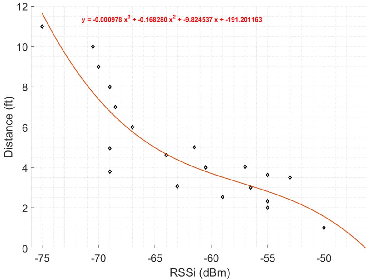
Figure 3.5: Look-up-table generated from the measured data in Edgar mine.
