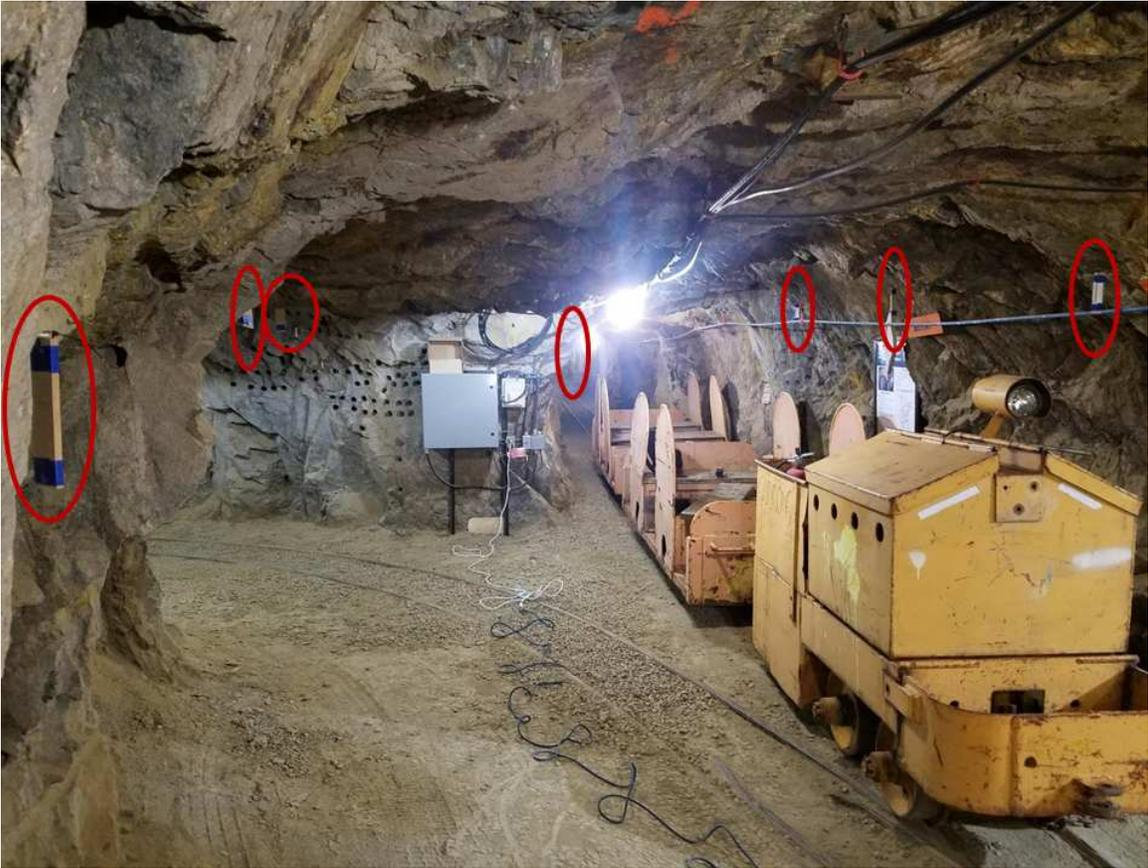
Figure 4.5: Picture of zone 3; an exemplary narrow intersection with the trolley acting as a large scatterer. The red ovals highlight the tags in view.
