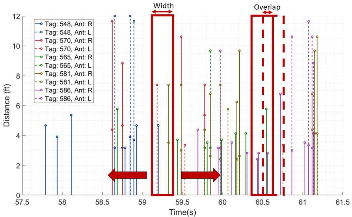
Figure 3.13: Distance from the user to each of the tags versus time. The look-up-table converted the RSSi to the distances shown in the figure. 'L' corresponds to the left antenna and the 'R' corresponds to the right antenna. The tag number corresponds to the last three digits of the tag ID. This figure also illustrates the swept window across the data. The window has a fixed width and is stepped through the code, in time, overlapping the next window by a time set by the user.
