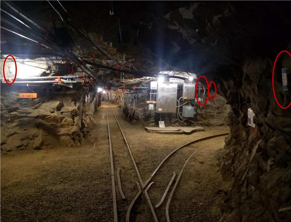
Figure 4.7: Picture of zone 8; an exemplary spacious intersection. The red ovals highlight the tags in view.
