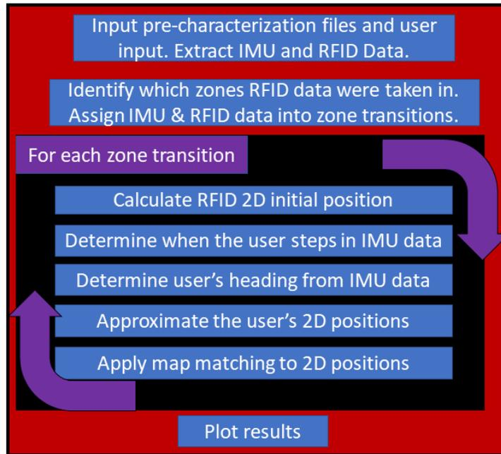
Figure 3.10: Flow diagram of the post-processing algorithm.
