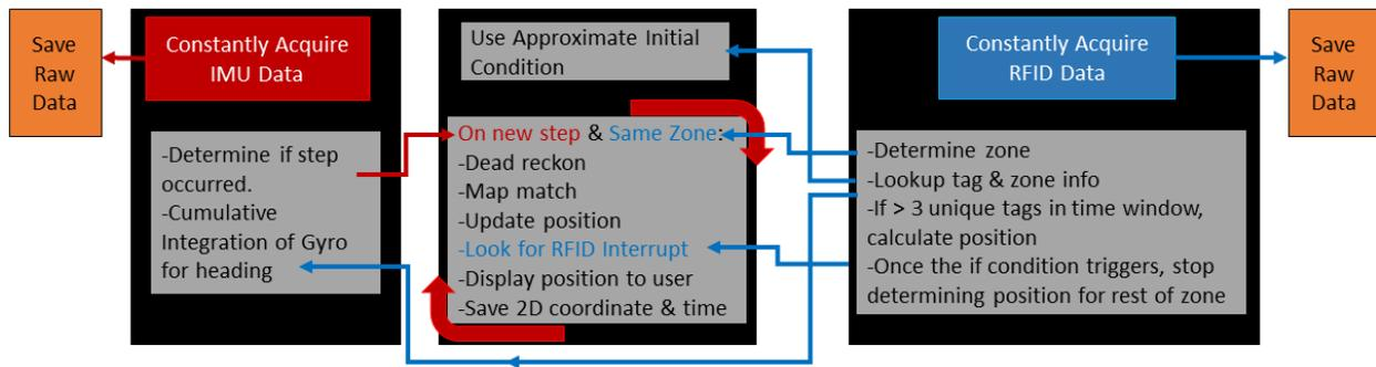
Figure 5.1: Block diagram for the proposed real-time algorithm.
