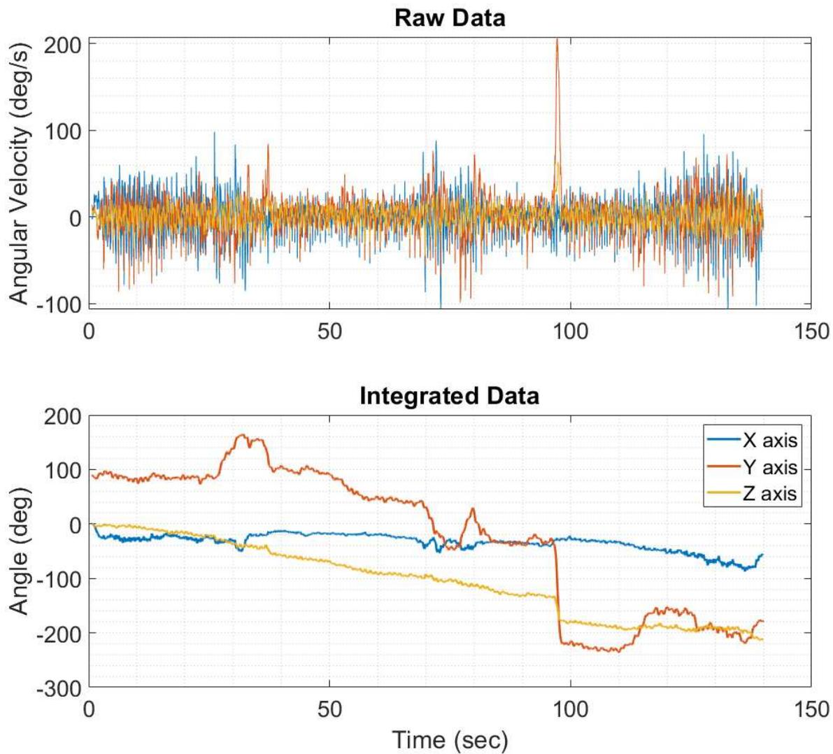
Figure 3.16: Raw data from the gyroscope for each axis (top) and the resulting heading after cumulative trapezoidal integration of the data (bottom). The X axis (blue), Y axis (orange), Z axis (yellow) corresponds to pitch, yaw, and roll, respectively. The user's yaw axis is used to calculate the heading for the IMU dead reckoning. Data shown are from the Edgar mine measurements.
