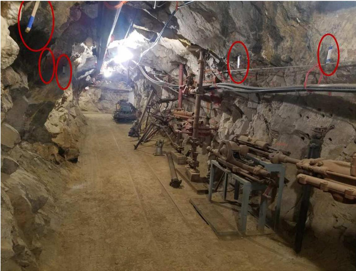
Figure 4.6: Picture of zone 6; a straight section full of mining equipment making it a complex scattering environment. The red ovals highlight the tags in view.
