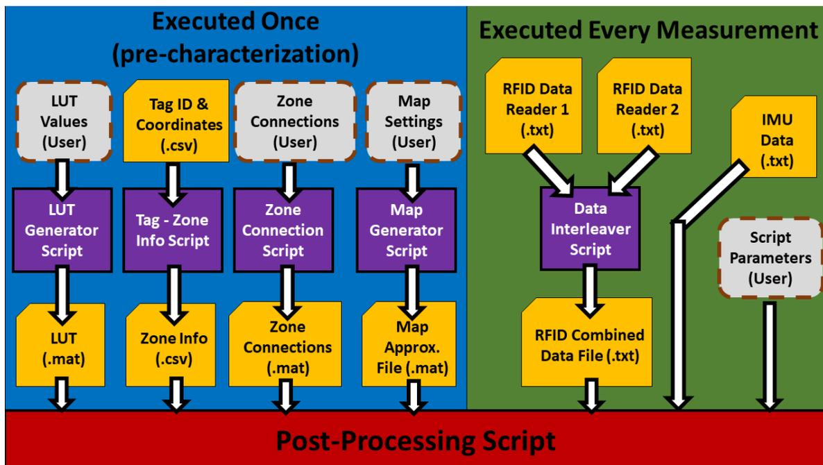
Figure 3.1: Flow diagram of all of the pre-processing scripts and files that feed into the post-processing script.
