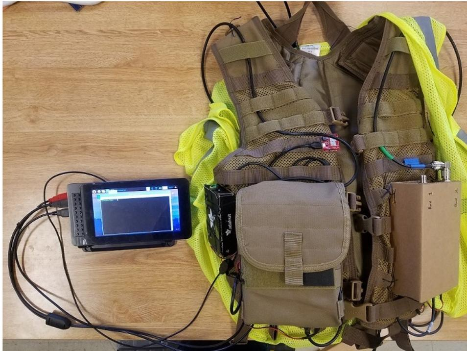
Figure 2.2: Complete wearable prototype. The vest contains two RFID readers, IMU, battery, and power circuit. The touchscreen contains the raspberry pi which connects to the power circuit, IMU, and RFID readers.
