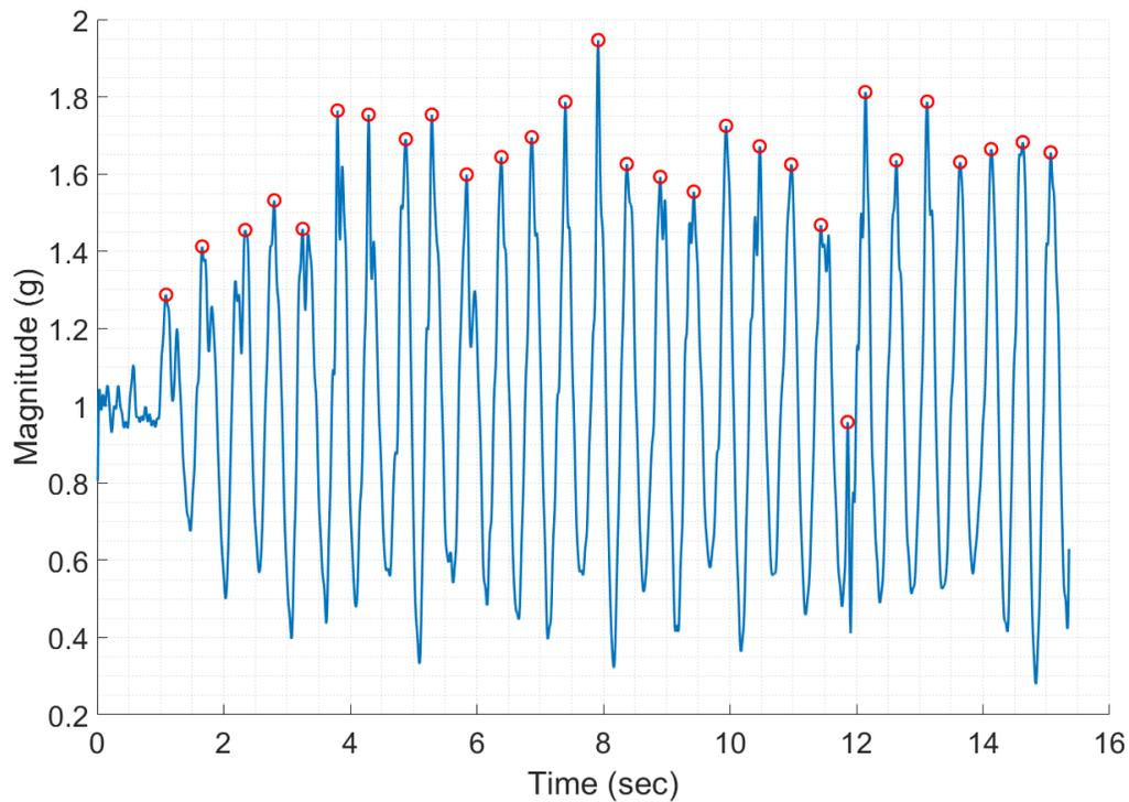
Figure 3.15: Magnitude of the time domain acceleration waveform after being filtered (blue). The red circles correspond to the peaks of the waveform that the peakfinder function [44] detected. Notice how for the first second the user is approximately stationary and no peak is detected. Data were taken from a portion of the IMU measurements during the Edgar mine experiment.
