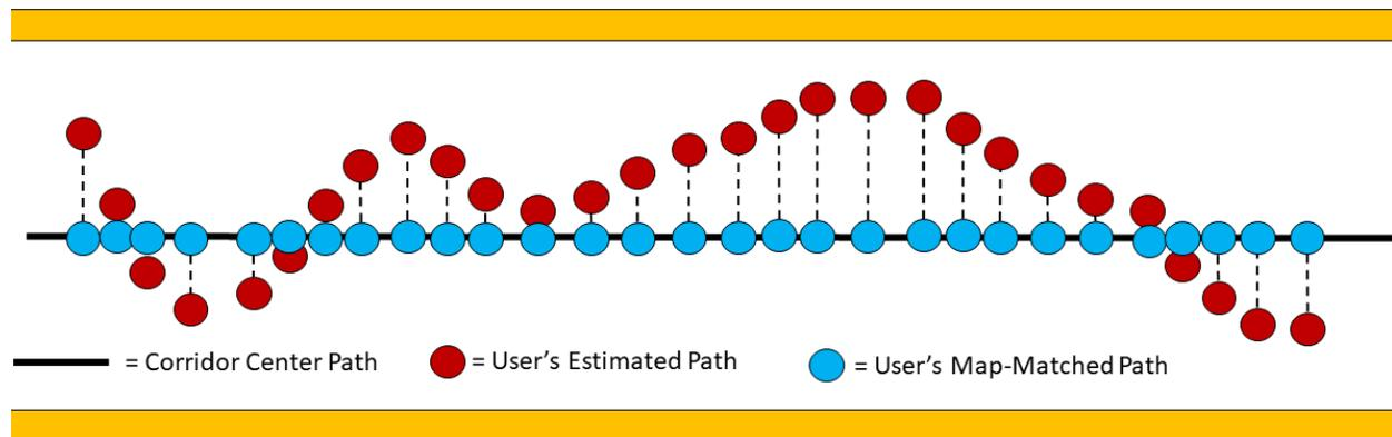
Figure 3.18: Diagram of point-to-curve map matching. All lateral position information is lost as the user’s estimated position is projected onto the center path.
