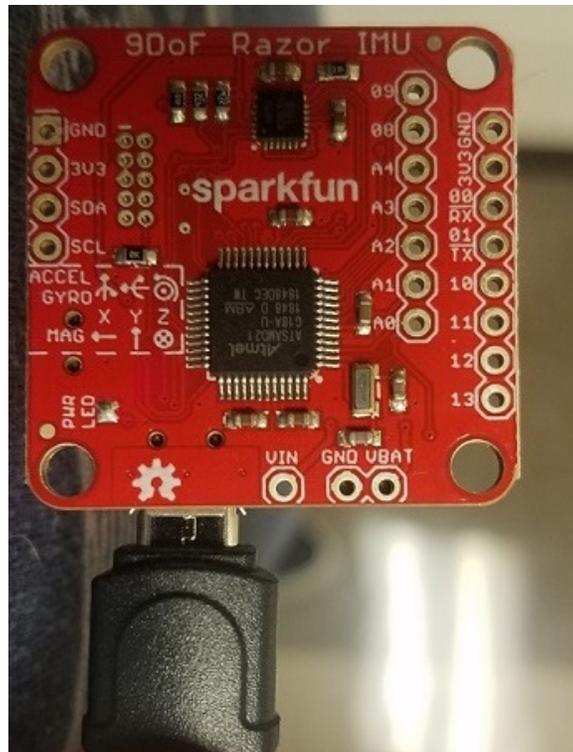
Figure 2.3: Sparkfun 9 DoF Inertial Measurement Unit.
