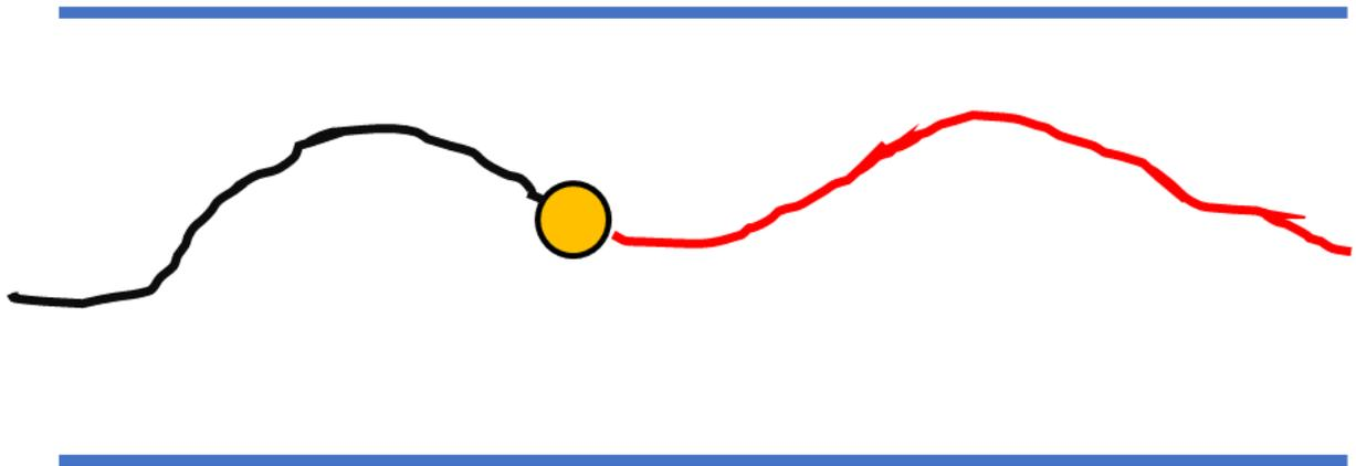
Figure 3.17: Simple diagram showing the initial position for the 2D function. The black line is the dead reckoned user position, from the IMU data, before the initial position. The red line is the dead reckoned user position after the initial position. All data still belongs to one zone.
